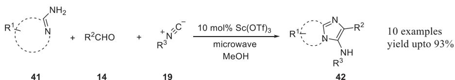
**Figure 3.16:** Microwave-assisted  $\text{Sc}(\text{OTf})_3$ -catalyzed 3 CC Ugi reaction for the formation of 3-aminoimidazoles.
